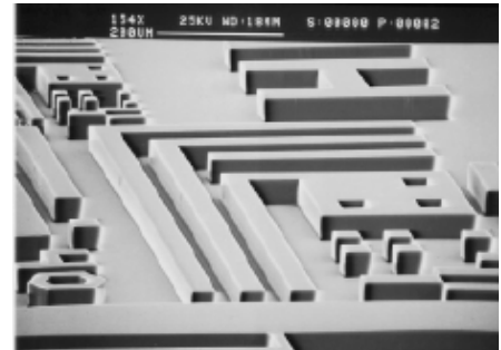
Contact print resolution mask in 40µm softbake film
