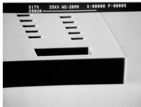
Via mask in 40µm softbake film
