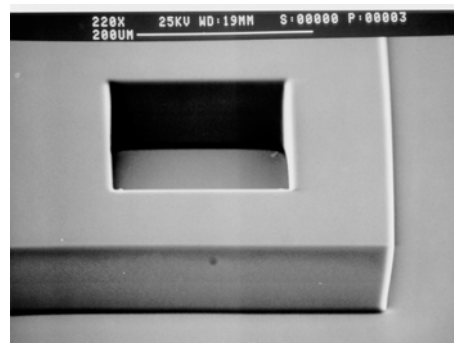
100µm via in 40µm softbake film
